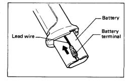
To prevent a battery short-circuit, tape the battery terminals or put the battery into a plastics bag. (Note: Never put two or more batteries into one plastics bag. Battery short-circuit may result.)
